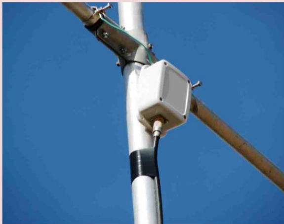
Feed point: 2-ferrite core with teflon coax balun
