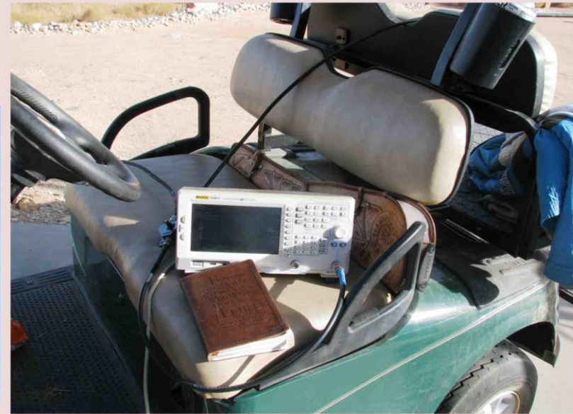
Spectrum analyzer with dual inputs: “candle” and antenna under test
