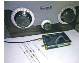
Figure 1 — All you need to test tuner loss into many loads, including an antenna.
